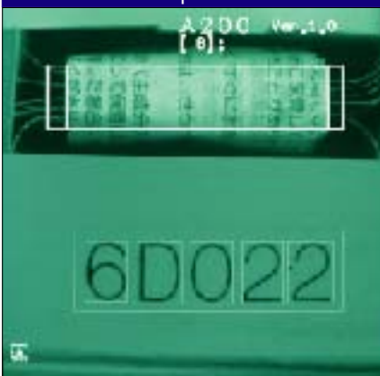
Inspection of stamped printing on boxes for cosmetics and pharmaceuticals.
