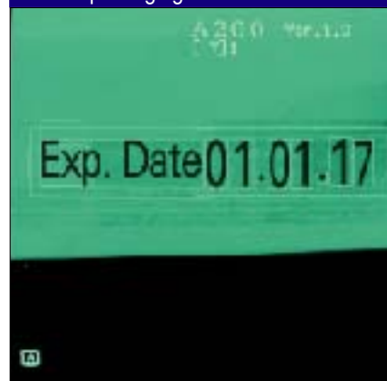
Inspection of "Use by" date information on film packaging for food.
