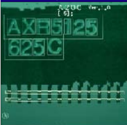
Inspection of printing and leads on connectors.
