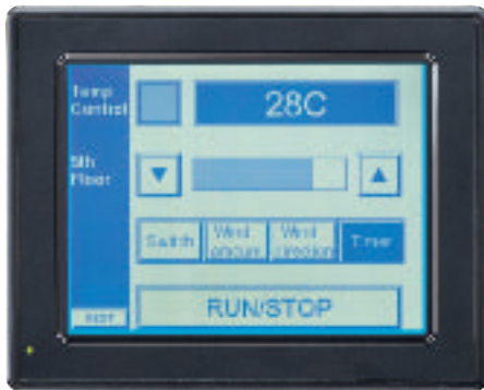
GT30M Bright and easy-to-read blue-mode LCD type.
